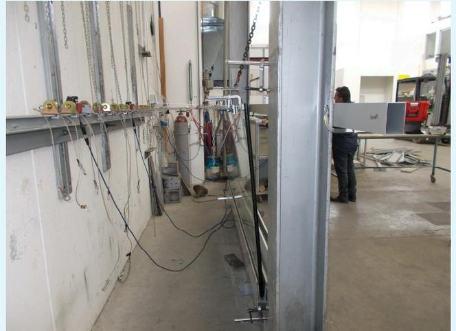
**Photographs of the sample during outward horizontal static loading test**
