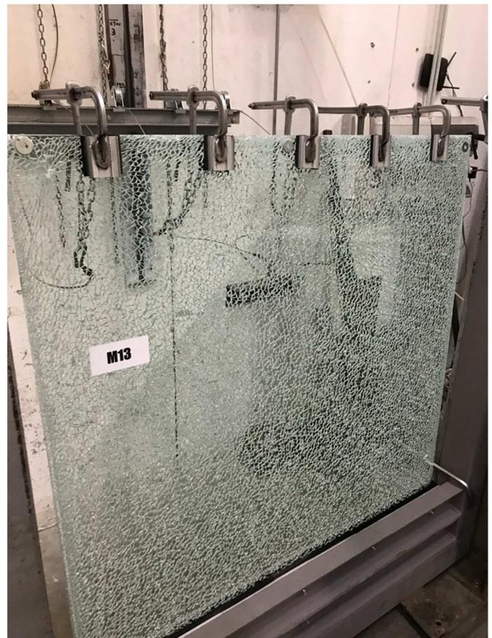
Photograph of the railing after breakage
