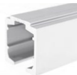
PCA-GT04 Guide Track Profile 580 cm | Length 1,248kg | Weight/meter Aluminium | Material Natural Anodize, Satin | Finish
