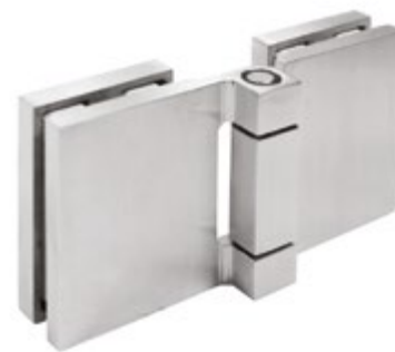
PCA-SH48 Glass - Glass Hinge 10mm | Glass Thickness 40 kg | Max. Weight Stainless Steel 304 | Material Satin, Polished, Black Anodize | Finish
