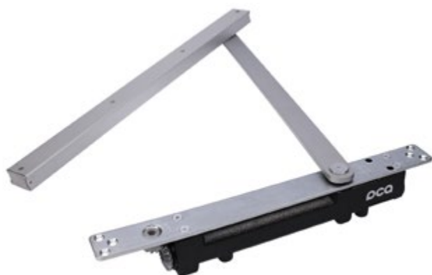
PCA-DC03 Concealed Door Closer 80 kg | Max. Weight Stainless Steel 304 | Material Natural Anodize | Finish
