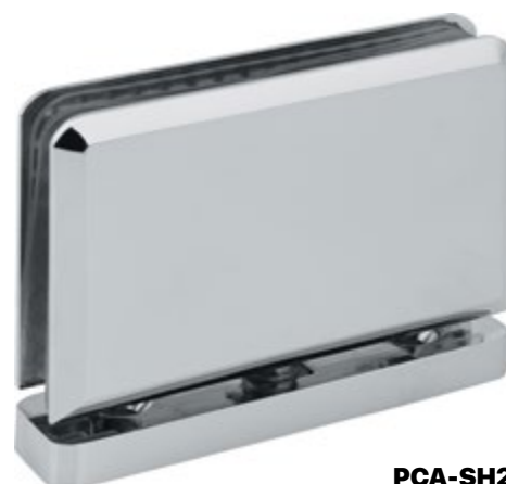
PCA-SH20 Top or Bottom Mount Pivot Hinge 8-10mm | Glass Thickness 45 kg | Max. Weight Brass | Material Satin, Polished | Finish
